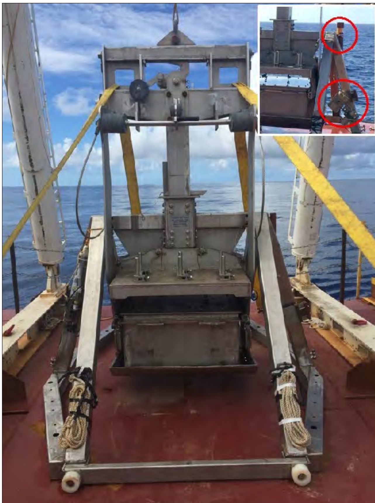
Figure 7.8 KC Denmark 0.75 m 2 box corer
