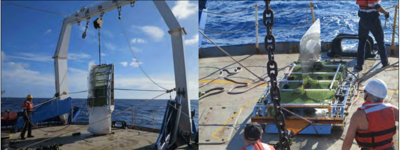
Figure 7.3 Photos showing the operation of the epibenthic sled collecting nodules during the NORI 2013 campaign
