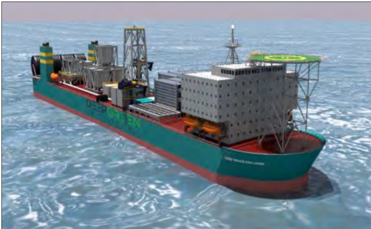
Figure 13.10 Collector Ship 1, production support vessel
